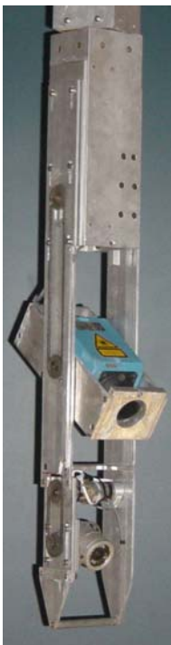
Close-up of Ferret tool showing the laser and laser tilt axis with borehole camera below.
