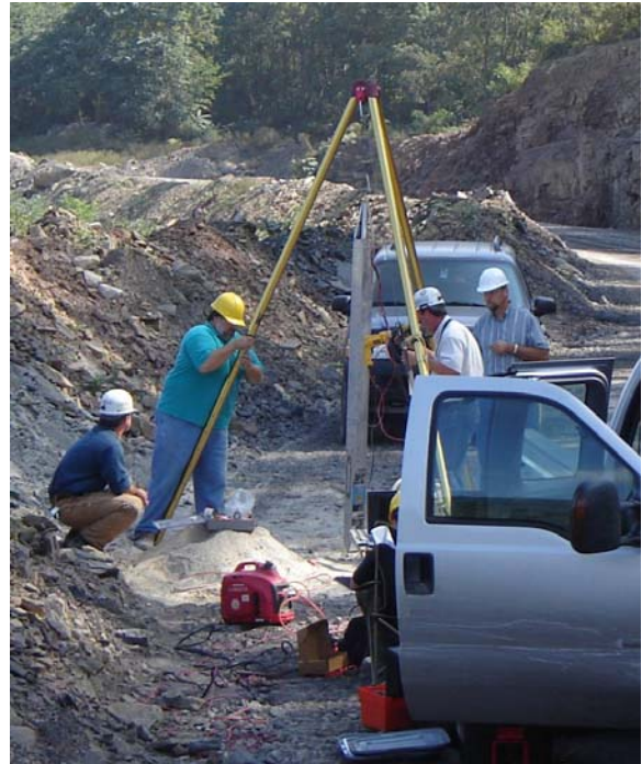
Close-up of Ferret tool and deployment at the Lots Branch site hanging from a tripod entering into an uncased hole – B18
